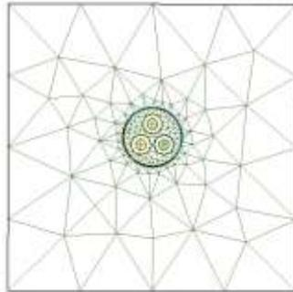
**Figure 44: example meshing for XVB cable**
