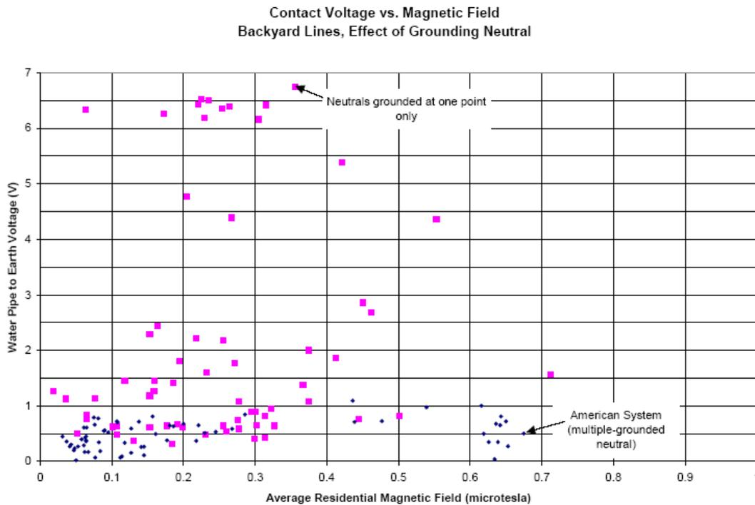
**Figure 24: Comparison between the American system and a system with the grounding of neutral at one point (EU).**
