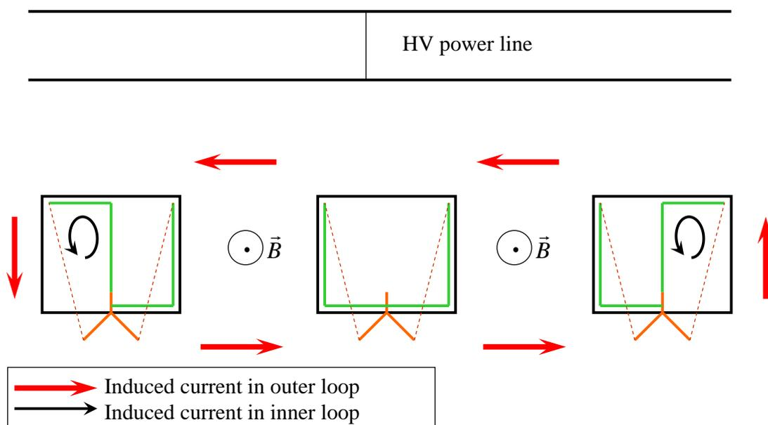
**Figure 18 : Scheme to explain the influence of a network of houses on induced currents level.**
